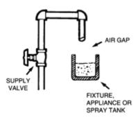
Used mainly on tanks and faucets, it is a gap between the pipe and the container. Requirements:
