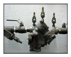
Used on high hazard buildings and is a combination of check valves and an air inlet allowing water from the private system to vent when City pressure drops.
