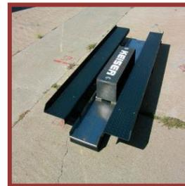
**Force Machine** – This unit consists of a steel track and a steel sled with plastic runners. The candidate swings the Dead-blow Hammer to strike the 158-pound Sled and move it down the track for a total of 3- feet.
